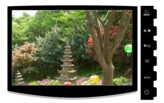
When OSD is not on the screen, push the **Brightness** ( ) button to adjust brightness.
